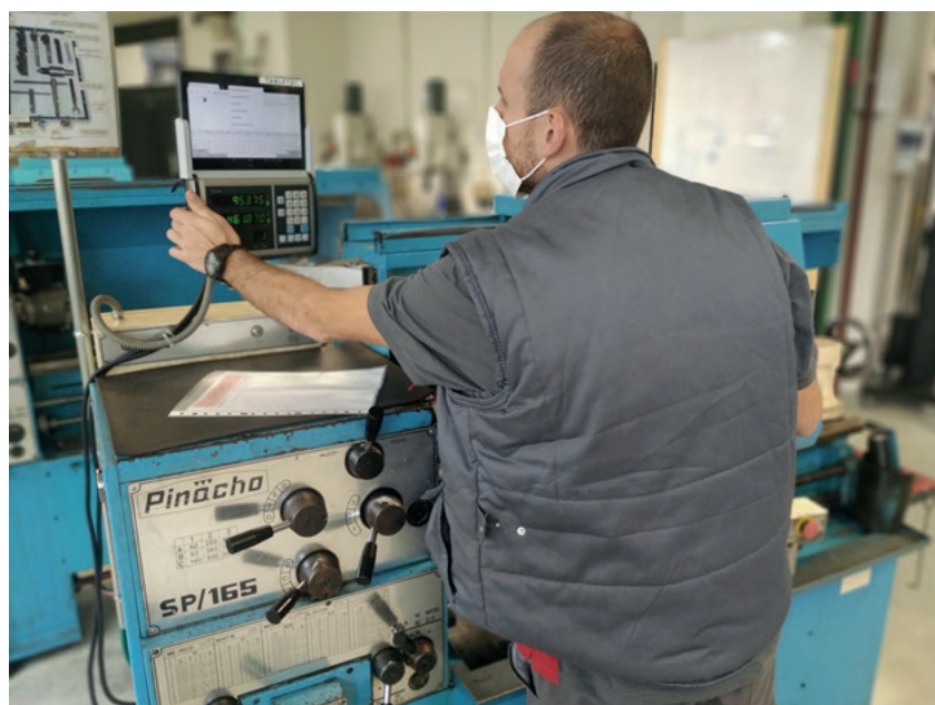
Figure 3: teacher using a digital process sheet made in the Odoo platform (ERP) in the digital touch device of a tuning machine.
