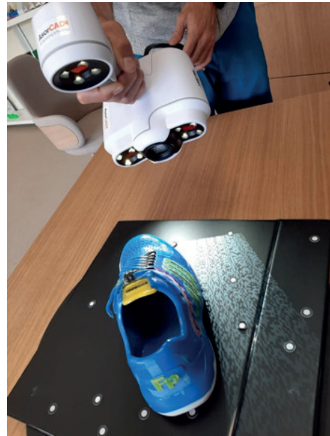
Figure 6: Scanning with Creaform Academia. Source: Tknika
