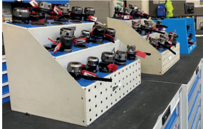
Figure 7: Tools classified by RFID system in Miguel Altuna's lab. Source: author's creation
