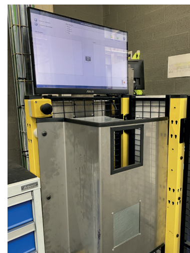
Figure 10: User and tool exit detector with RFID system in Miguel Altuna's lab. Source: author's creation
