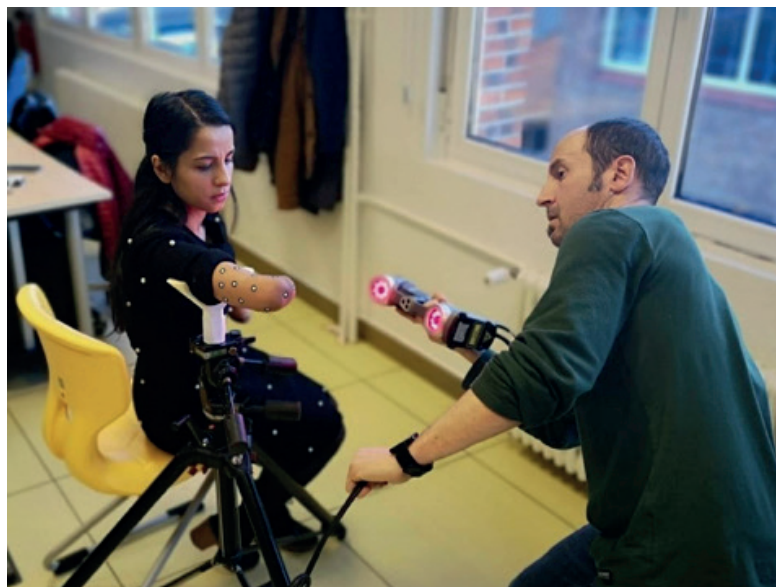
Figure 7: Scanning Maria's arm with Creaform Handyscan 700 scanner. Source: Tknika
