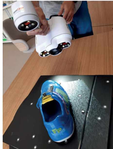
Figure 6: Scanning with Creaform Academia. Source: Tknika
