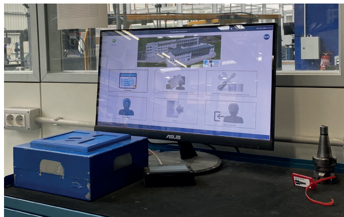
Figure 9: Consultation device using an RFID system within the intelligent warehouse of Miguel Altuna's lab. Source: author's creation
